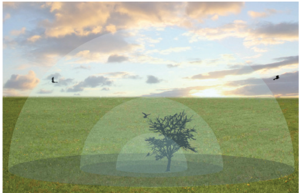
Schematic representation of how masking reduces an animal’s listening area. As background sound levels increase, the area in which the perched bird can hear biologically significant sounds, represented by the domes, is reduced. The intensity of masking, as measured by listening area reduction, depends upon the characteristics of the biological signal, the noise, and the animal’s auditory system. Image by Ted E. Dunn
