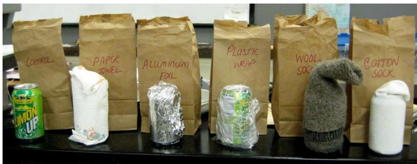
*Teacher Note:* All of the materials in the demonstration can be considered insulators to some extent because they all performed better than the control. However, wool and plush paper toweling are the best insulators because they trap air and prevent the air from moving around. In fact, paper is made up of dried up hollow cells from plant matter allows for many pockets of trapped air. Several real-world examples of insulators students may be familiar with include:
