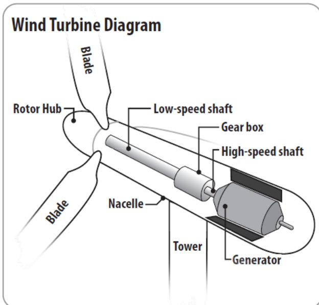
The wind blows and pushes against the blades on top of the tower. The blades catch the wind and spin the rotor.
